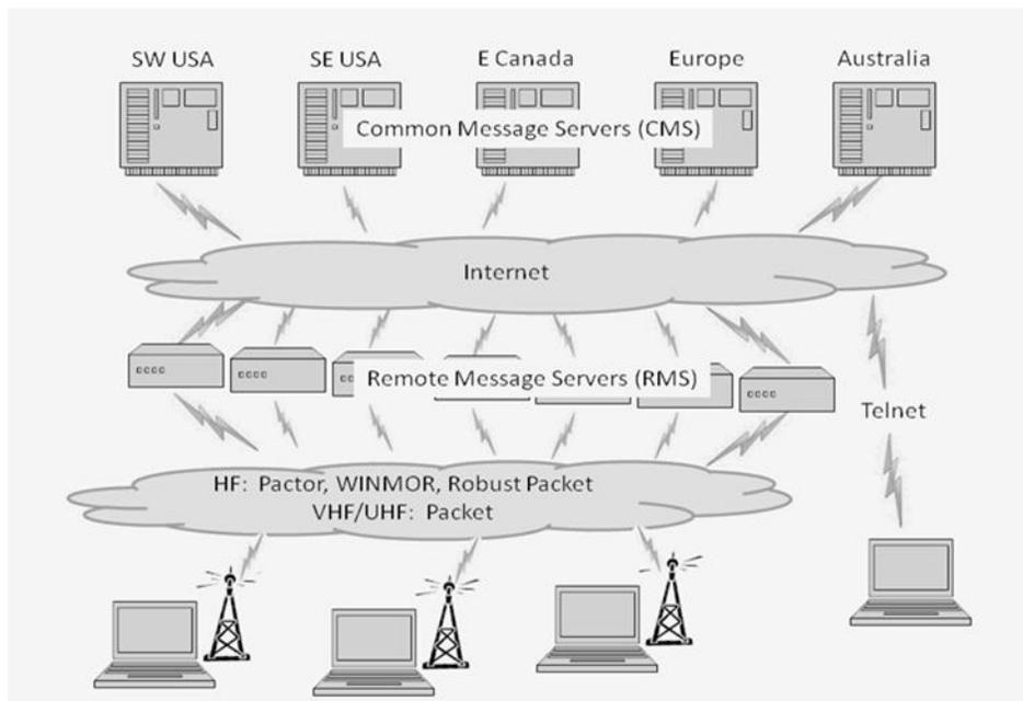
The Winlink system consists of a group of Common Message Servers (CMS) placed at various locations around the world. These servers connect via the Internet to Radio Message Servers (RMS) in many geographic locations to form a star network configuration. The Radio Message Servers are the VHF, UHF, or HF RF gateway into the Winlink system. The final component is the client computer (i.e., your computer) which runs software to send/receive messages through your radio.
