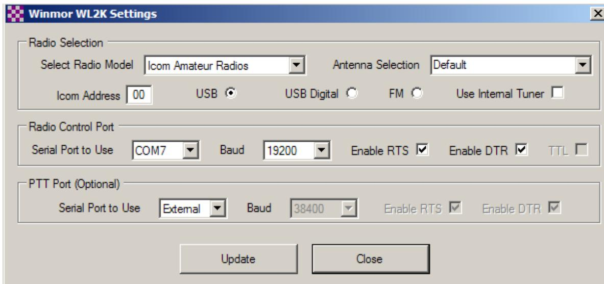
Open the “Select Radio Model” list and select the entry that is closest to the type of radio you have. Set the Radio Control Port fields to match the COM port and baud rate of your radio control interface. Set the PTT Port option to “External”. If you don’t have the ability to automatically control your radio, you can still use RMS Express. Just manually tune to the “dial frequency,” and set USB SSB mode. Click Update to close the setup screen.
