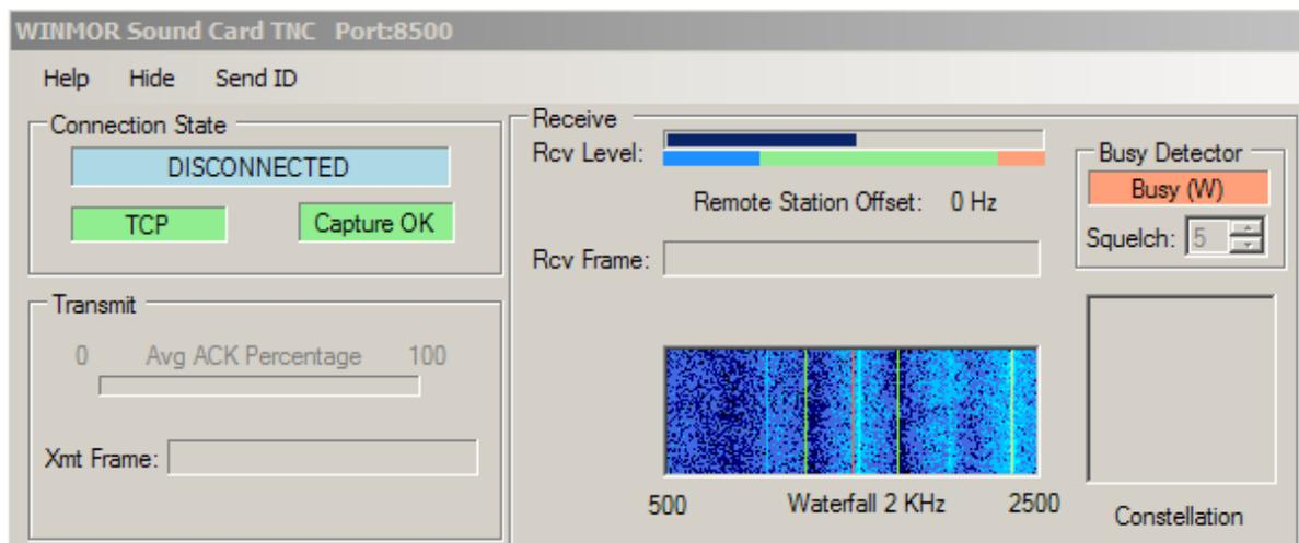
The "Busy Detector" on the TNC display should tell you if the channel is busy or clear, but it is often confused by noise, so it's best to look at the waterfall display to see if a signal is visible. If the channel is busy, either wait for the other station to finish or select a different channel.
