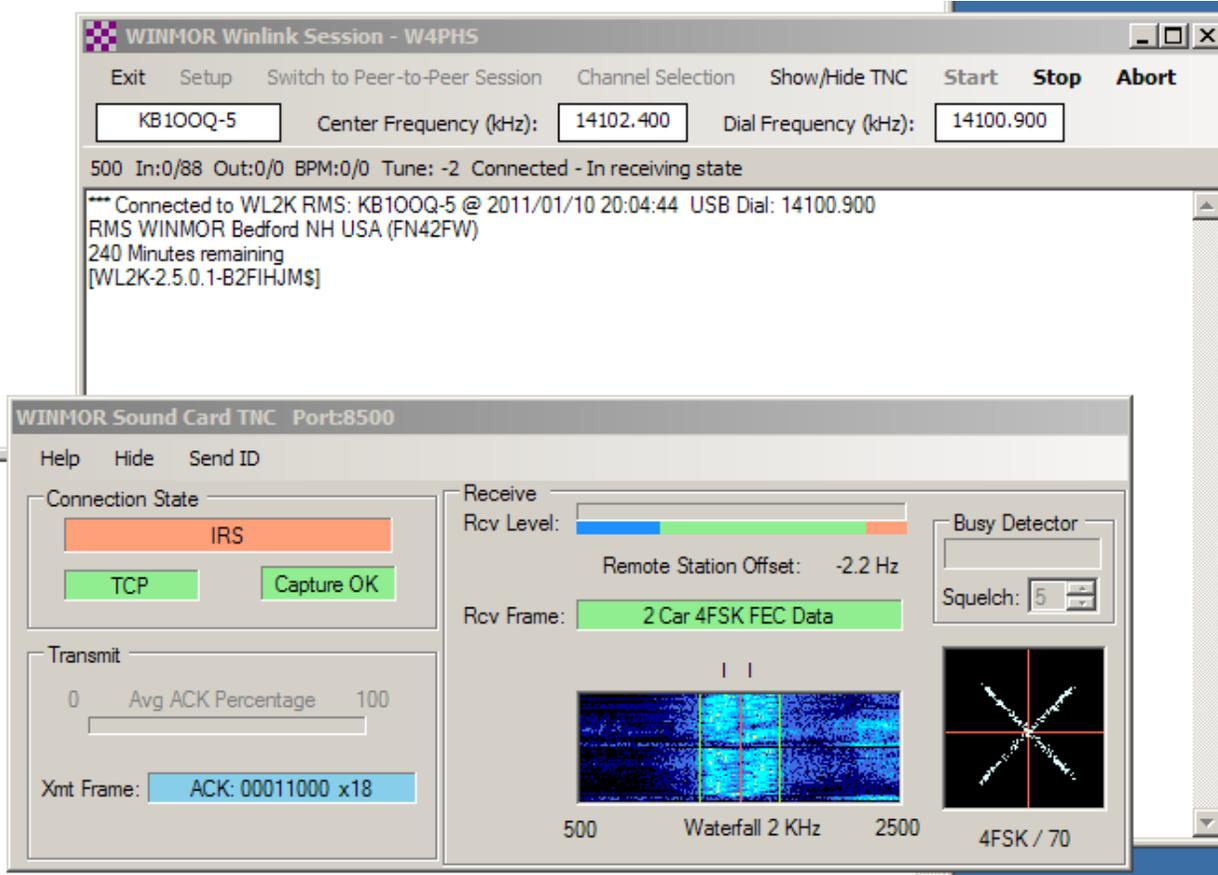
If you can't connect, try a different channel. If you do connect, watch the "Rcv Level" bar at the top of the TNC screen to make sure your received audio signal level is in the green zone. If it isn't, adjust the "RX" knob on the SignalLink to get it in the green region.
