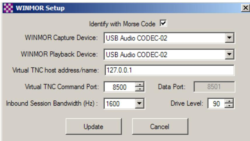
Select the sound card entry corresponding to the SignalLink in the WINMOR Capture and Playback fields; it will be labeled “USB Audio CODEC”, but the number at the end may be different. For ham operation, check the box “Identify with Morse Code”. Leave this box unchecked for MARS operation. After you finish filling in the soundcard information, click the “Update” button to save the information and close the screen.
